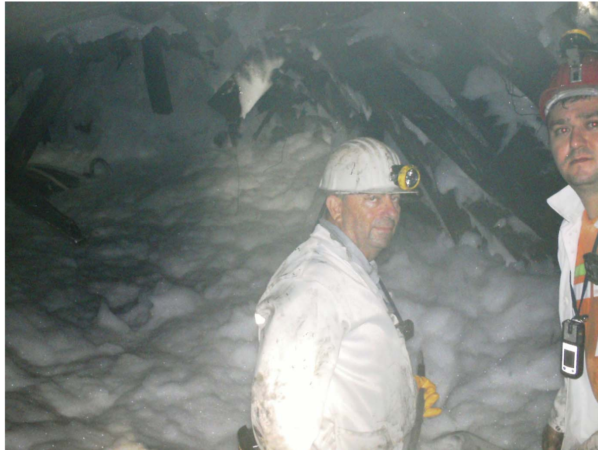
Result of Phase 2 : The head gate Kalin Damar is inundated with foam, ventilation engineer and assistant
