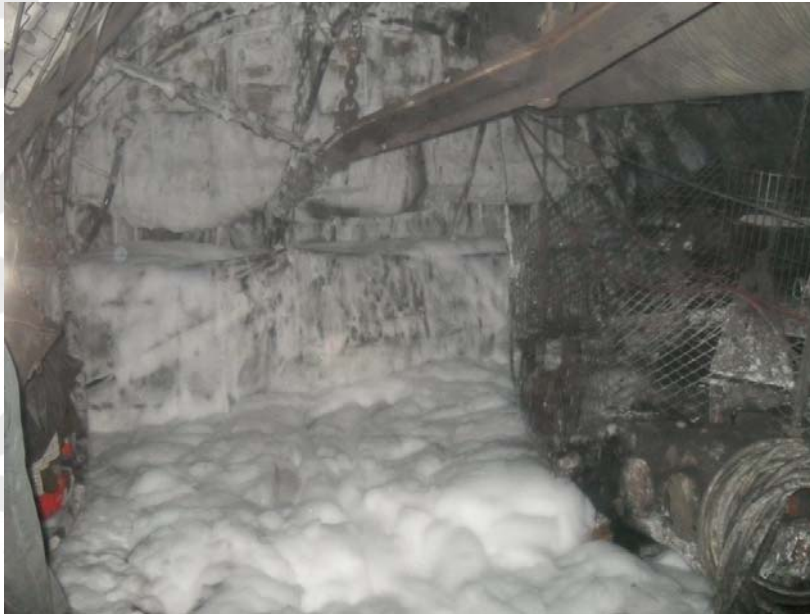
In order to reduce the oxy-reactivity of the coal the goaf is covered with a rather „dry“ foam.
